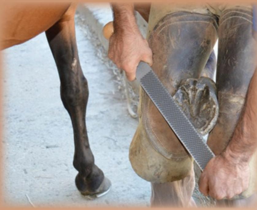
All Vallorbe horse rasps are manufactured of high carbon steel, with a service life almost twice as long as its competitors, a constant quality and a rasp side
